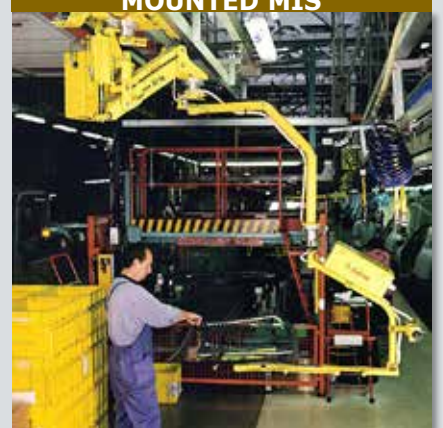
OVERHEAD TROLLEY MOUNTED MIS
